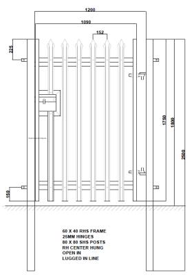
Palisade Fencing Gate Configuration
